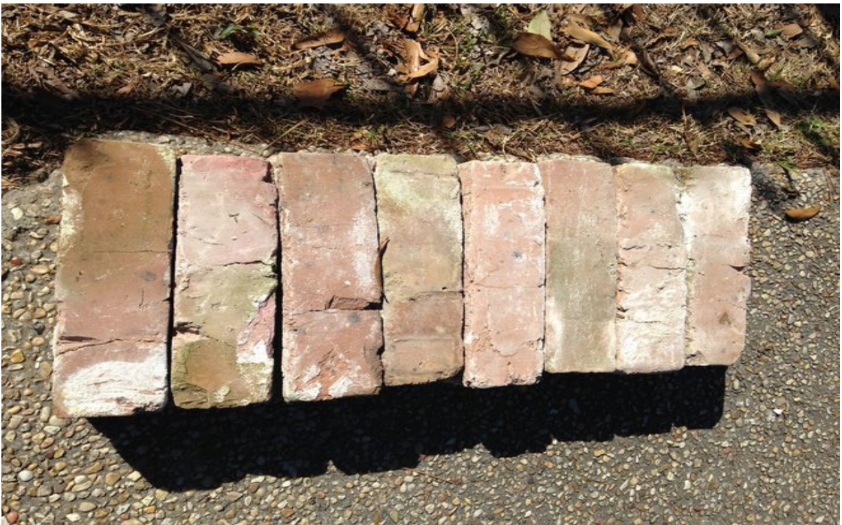
Figure 65. New Orleans lake brick: hard, tan bricks made from clay from Lake Pontchartrain and St. Tammany Parish.
