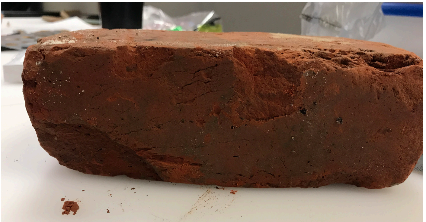
Figure 64. New Orleans river brick: soft, red brick made from clay from the banks of the Mississippi River.
